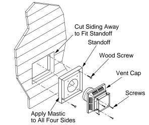
Figure 11 - Installing Siding Standoff
